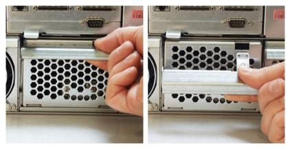
2. Press the release button and pull the handle downward as shown above.
